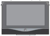
Keep the button under the wall holder pressed. Tilt the flat panel screen with the other hand into the desired position, then let go of the button. The angle of tilt is retained.
